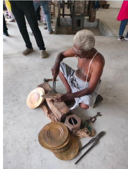
Artisan dividing the plate using mold divider.
